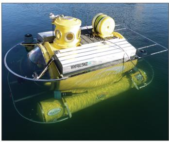
navigational and sonar equipment, of operating around the clock in low visibility and varying weather conditions, making her crews able to conduct timely, efficient surveys of the marine environment. In addition to a standard suite of navigational and sampling equipment, including a manipulator arm, multibeam sonar, and high-def imaging capabilities, *Antipodes* is fully configurable to fit the most complex data collection needs of the research and commercial community.
